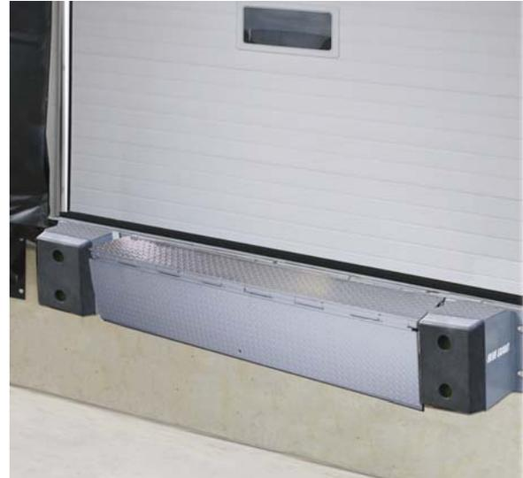
Mechanical EOD is activated by the operator pulling the lip and deck into the raised or extended position. The lip is then lowered down onto the trailer bed. After the trailer departs, the EOD retracts into its lowered position behind the bumpers.
