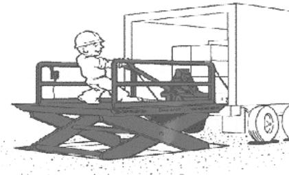
3) **Lifting Speed.** The lifting speed is determined by the size and capacity of the elevating dock and the size of the power pack. Power packs are available in virtually any horsepower. Selecting a small power pack to save money can result in a substantial loss of efficiency. Specify the desired speed at which you want the lift to operate. A recommended time for full lift is 20 - 30 seconds. Lowering times should also be considered.
