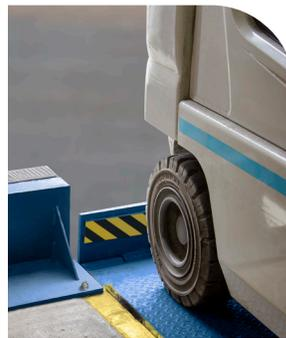
The Dock Lip Safety Barrier is an economical alternative to the XDS and an additional line of defense against worker injury and property damage. When the dock leveler is in the parked position, the steel barrier extends 5" (127mm) above the deck surface, preventing warehouse traffic from rolling off the edge of the dock.
