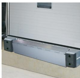
Edge-of-dock levelers are ideal for locations that cannot support the installation of a pit leveler. These compact and self-storing units are easily applied to a dock face, and provide a sturdy bridge between the dock and the trailer. Edge-of-dock levelers are available in both hydraulic and mechanical designs.
