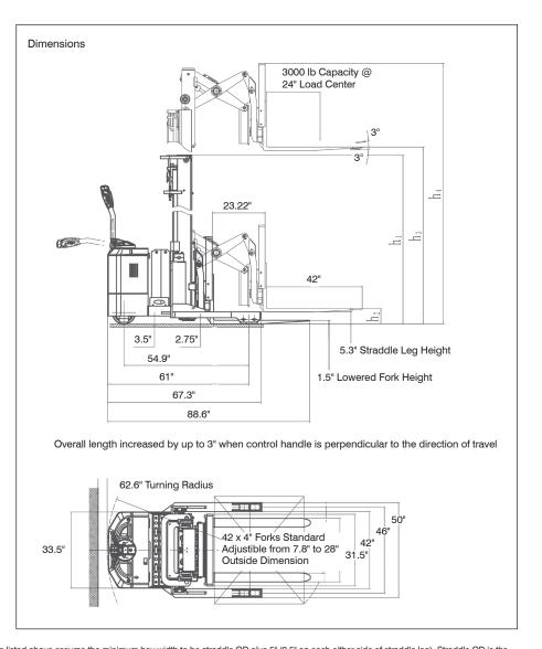
Note: Aisle dimensions listed above assume the minimum bay width to be straddle OD plus 5" (2.5" on each either side of straddle leg). Straddle OD is the load width plus 10". Truck performance may vary due to application requirements and changes in model design.
