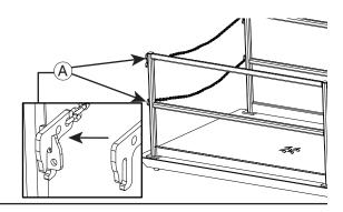
10. If present, verify that any entry (or building) side lip is manually raised and chained, or the hydraulic lip is fully raised and chained.
