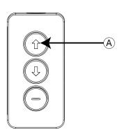
12. When deck is level with or slightly above trailer bed (by one (1) in. (25.4 mm) to two (2) in. (50.8 mm)), release the button. This provides a gentle lip slope that reduces crowning/obstructions or severe gaps. If present, the rolling stop guard will deploy.
