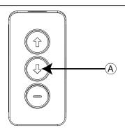
10. When deck is level with the building side floor or stops lowering, release the button.
