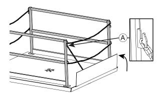
Remove entry (or building) side personnel restraint chains. If present, do the same for any interlock door or gate.
