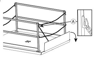
Remove the exit (or trailer) side personnel restraint chains. If present, do the same for any interlock door or gate on the exit side.
