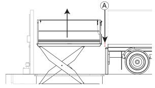
13. On the exit side, unchain and manually lower the lip, or unchain and lower the hydraulic lip onto the trailer bed.
