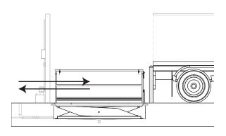
14. If transfer complete, reattach entry (or building) side personnel restraint chains. If present, do the same for any interlock door or gate on the exit side.
