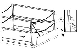
NOTE: Verify that the deck lip has a minimum of four (4) in. (102 mm) of overlap with the trailer bed.
