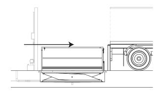
7. Verify that the load is positioned on the deck between where the scissor legs will be in the raised position AND in the lateral (left/right) center of the deck. The center of gravity of the load must be between the two scissor legs otherwise deck tipping may occur during raising of the lift.
