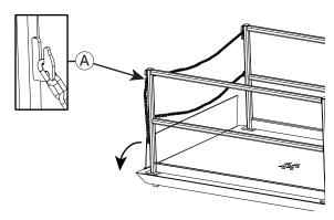
12. Remove entry (or building) side personnel restraint chains. If present, do the same for any interlock door or gate on the entry side.
