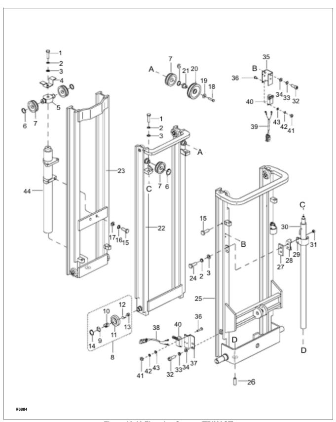
Figure 12-10 Elevation System (TRIMAST)
