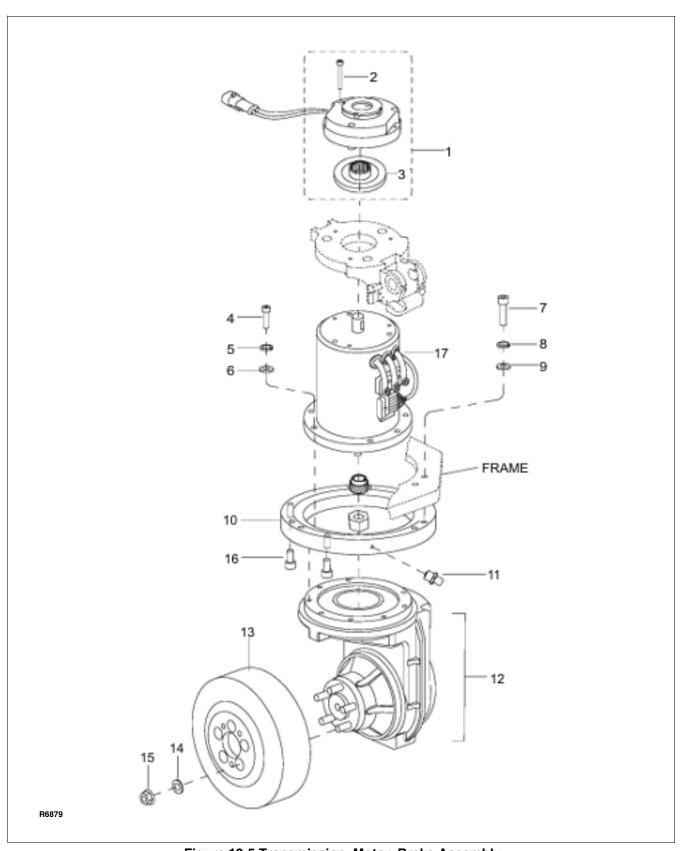
Figure 12-5 Transmission, Motor, Brake Assembly
