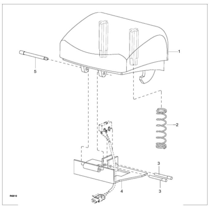
Figure 12-4 Emergency Reverse Switch Assembly
