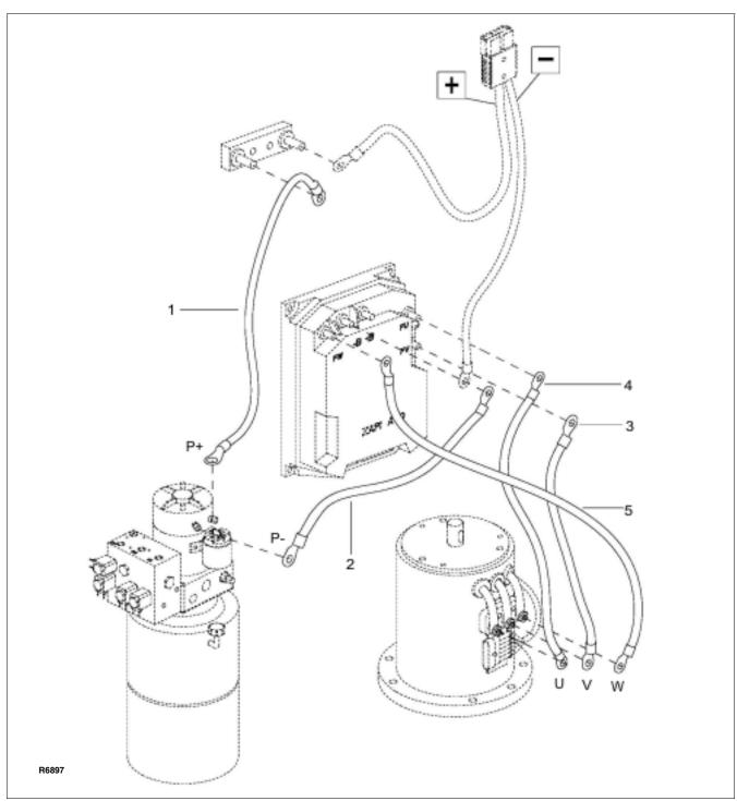
Figure 12-26 Wiring Cables
