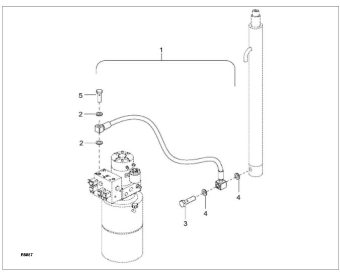
Figure 12-15 Hydraulic System (Telescopic)
