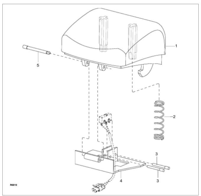
Figure 5-3 Emergency Reverse Switch Assembly
