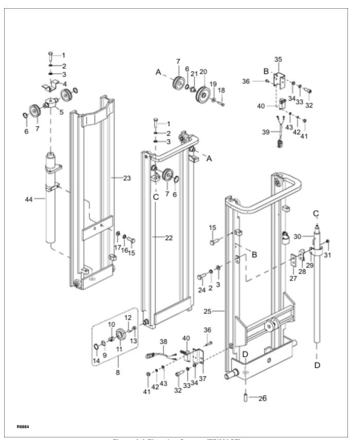
Figure 9-6 Elevation System (TRIMAST)
