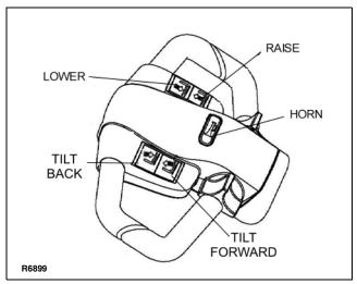
Figure 2-4. Pushbutton Switches
