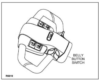
Figure 2-6. Belly-Button Switch
