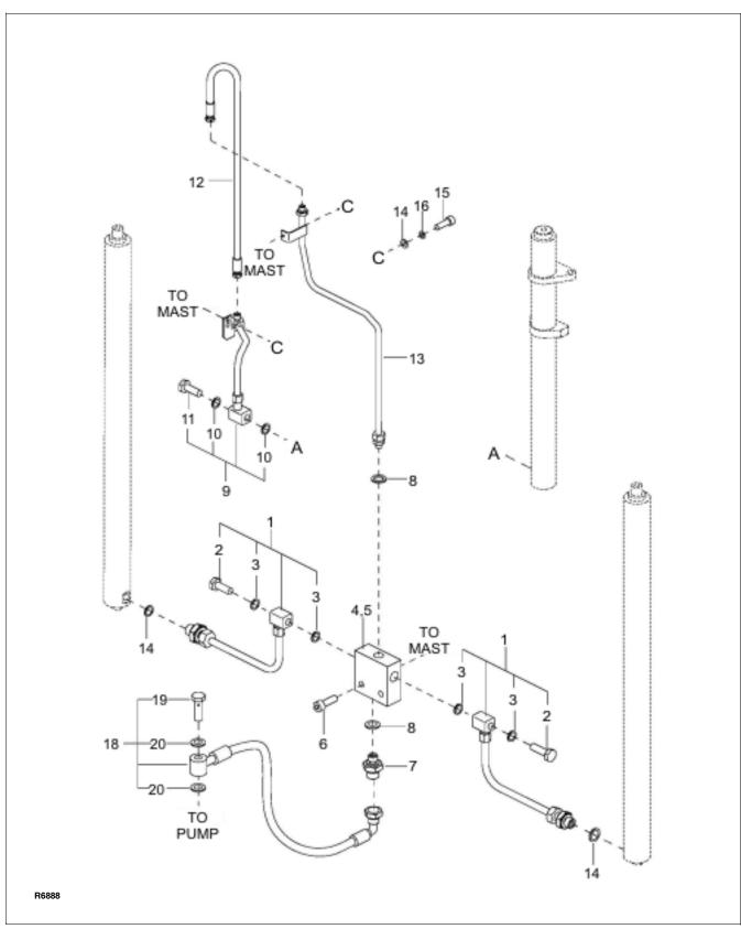
Figure 12-16 Hydraulic System (TRIMAST)
