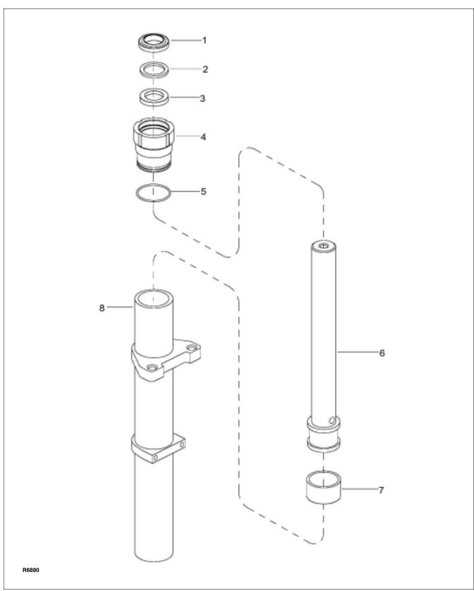
Figure 9-7 Free Lift Cylinder (TRIMAST)
