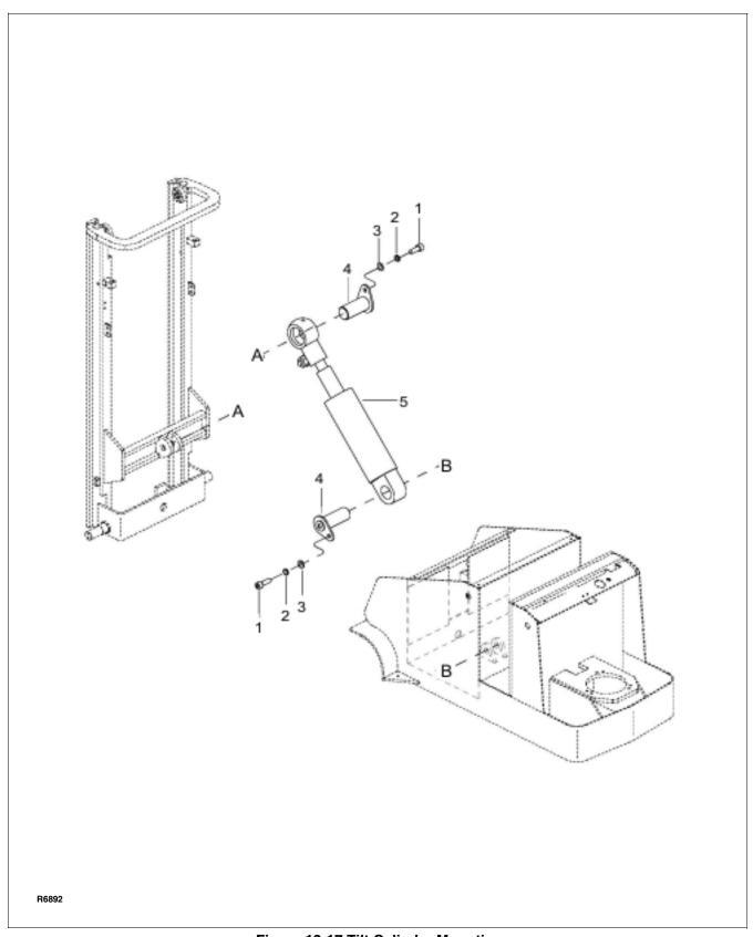
Figure 12-17 Tilt Cylinder Mounting
