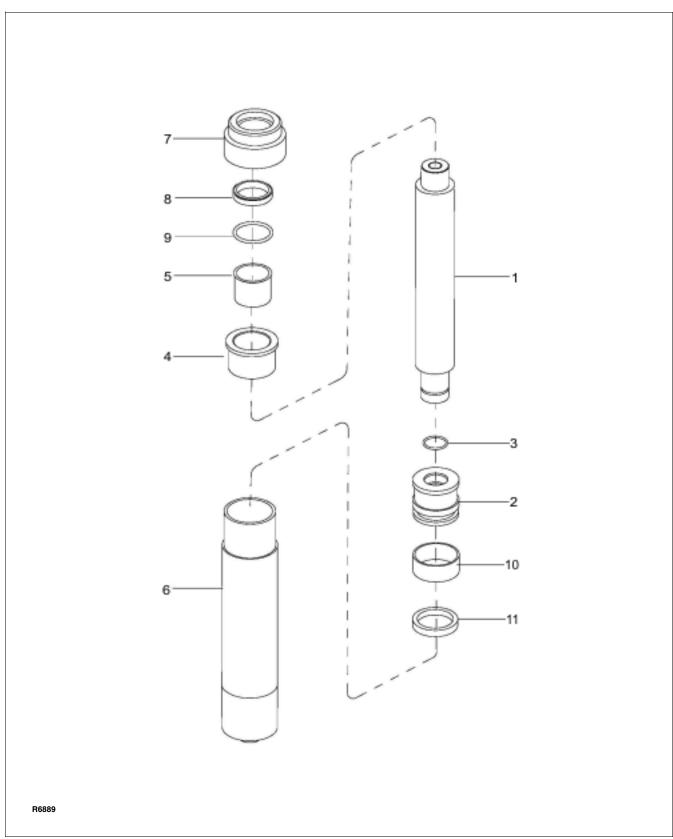
Figure 12-18 Lift Cylinder (Telescopic)
