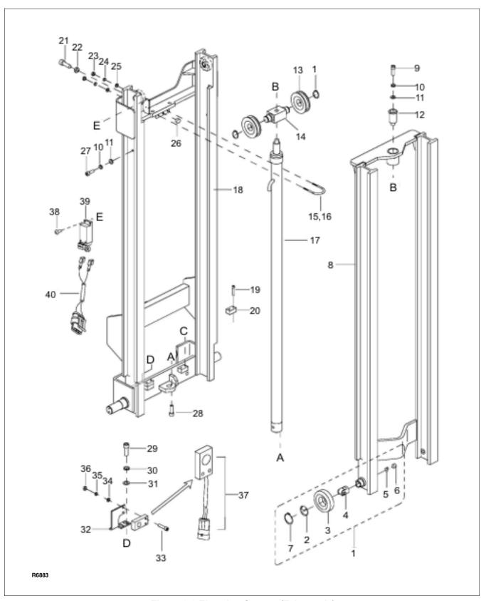
Figure 8-2 Elevation System (Telescopic)
