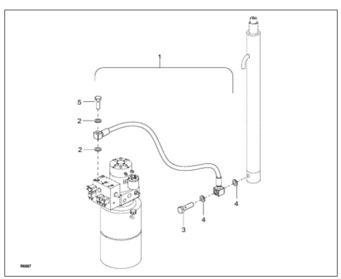
Figure 9-2 Hydraulic System (Telescopic)
