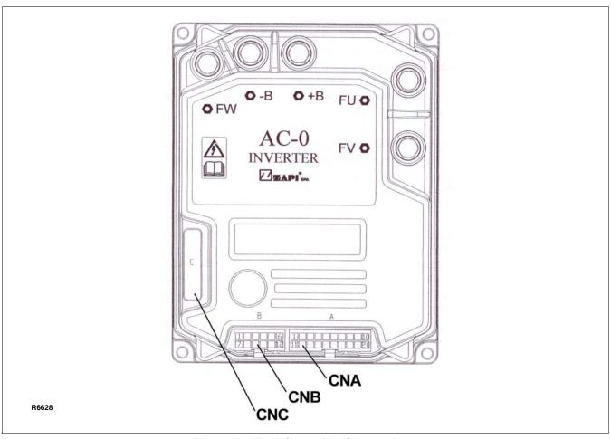
Figure 4-6 Zapi Controller Connections
