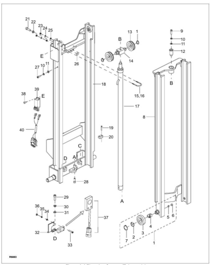
Figure 9-4 Elevation System (Telescopic)
