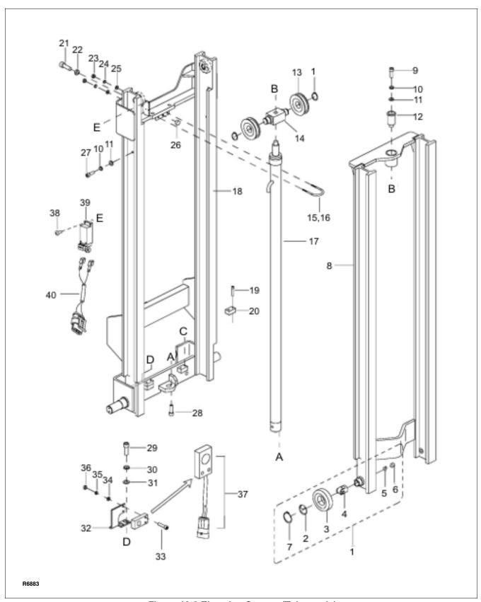
Figure 12-9 Elevation System (Telescopic)
