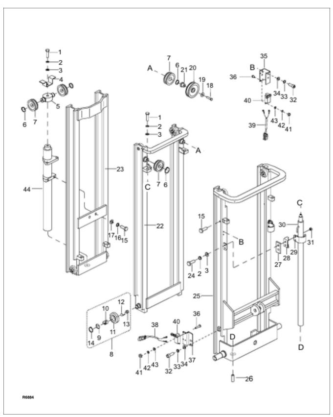
Figure 8-3 Mast (TRIMAST)
