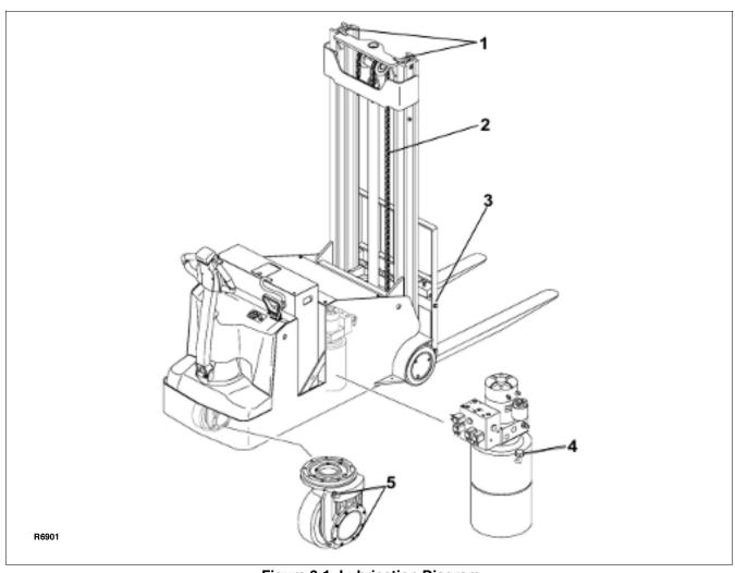
Figure 3-1 Lubrication Diagram
