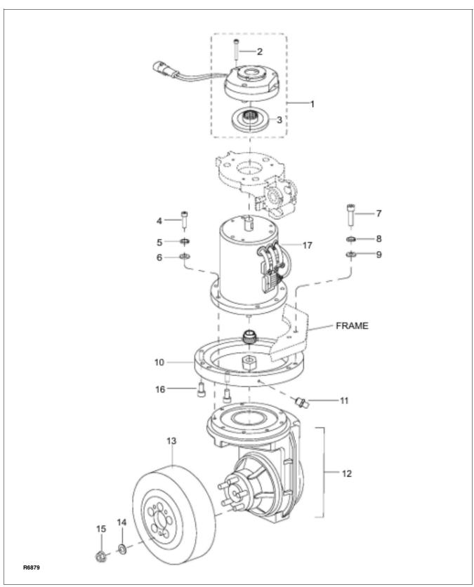
Figure 10-3 Transmission, Motor, Brake Assembly
