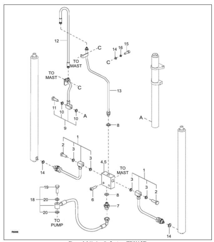
Figure 9-3 Hydraulic System (TRIMAST)
