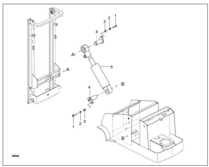
**Figure 9-9 Tilt Cylinder Mounting**
