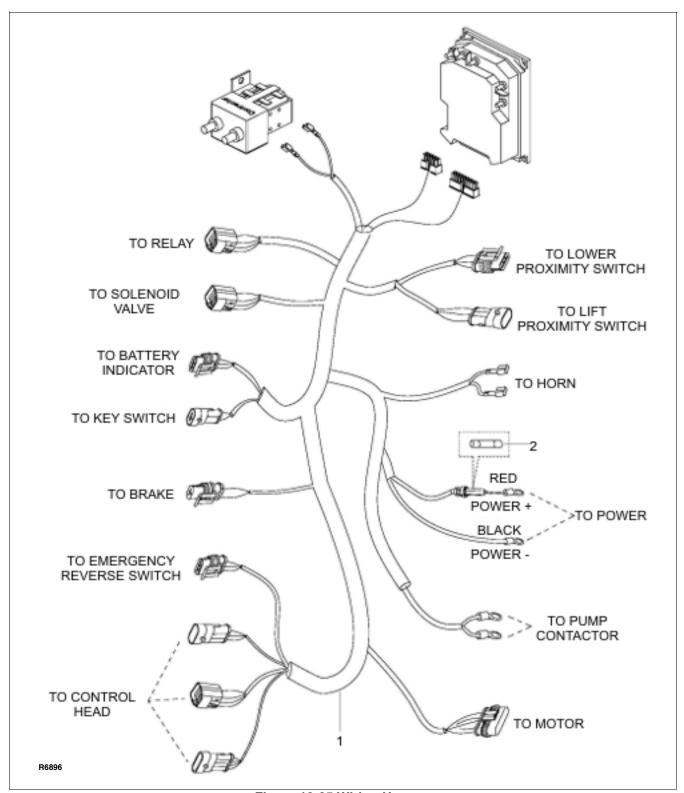
Figure 12-25 Wiring Harness
