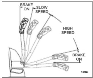
Figure 2-5. Brake Actuation
