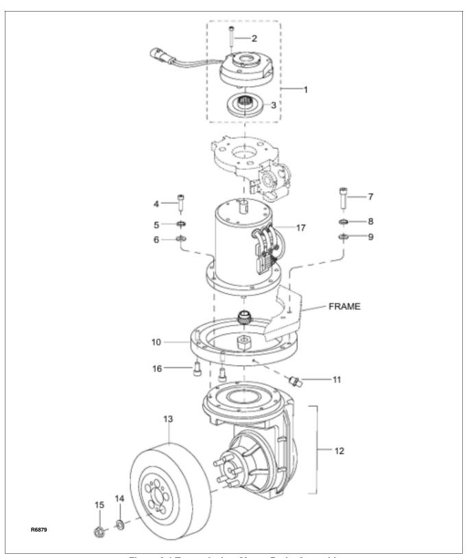
Figure 6-1 Transmission, Motor, Brake Assembly
