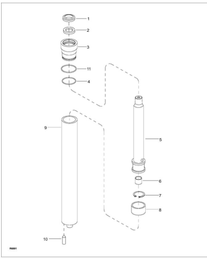
Figure 9-8 Secondary Lift Cylinder (TRIMAST)
