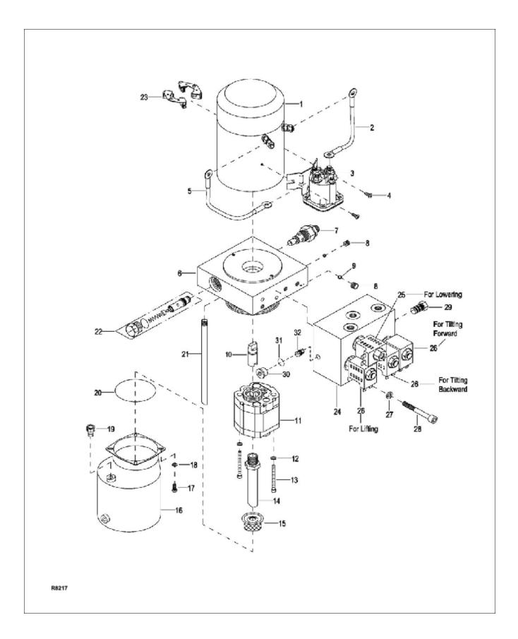
Figure 12-14 Pump & Motor - Used from serial number 324200459
