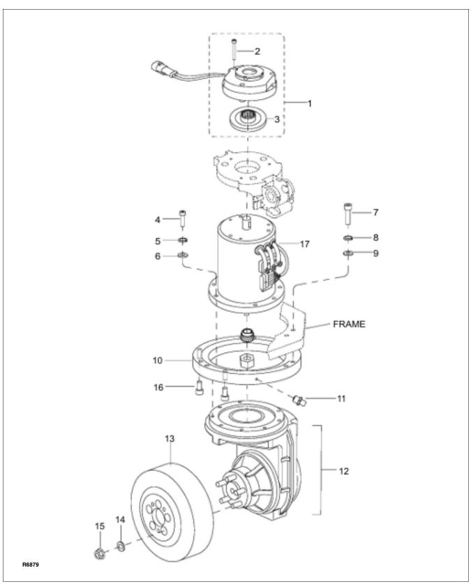
Figure 7-1 Transmission, Motor, Brake Assembly
