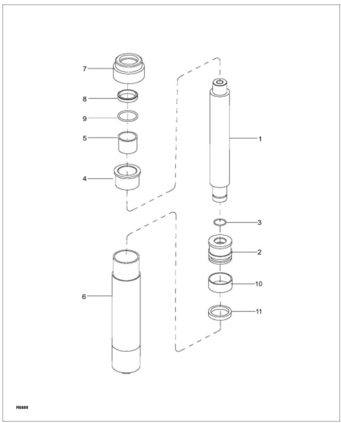
Figure 9-5 Lift Cylinder (Telescopic)
