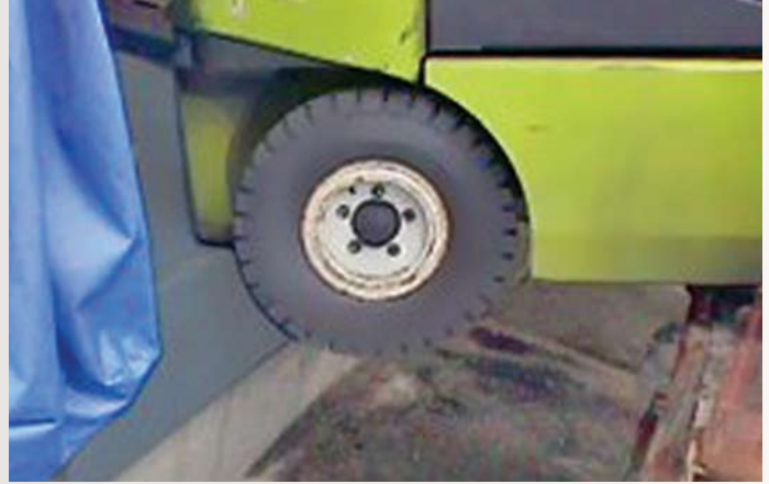
"Trailer creep" occurs when a trailer gradually shifts away from a loading dock, despite being parked there. Motion inside the trailer—usually caused by the stopping and starting of lift trucks inside—causes a gradual slide of the trailer away from the dock.
