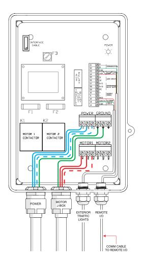
Blue Genius™ control station wiring layout for 115V single phase only.
