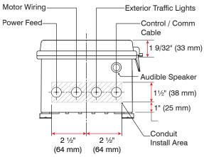
**NOTE:** Install high power conduit from the bottom of the control panel. Do not ty-wrap low voltage cable(s) to the outside of high voltage conduit(s). Maintain a minimal 1" (25mm) separation between the two.
