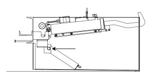
Push the hook cylinder assembly back and into its trunnion. The tilt cylinder will enter its trunnion shortly before the hook cylinder does. As the hook cylinder enters its trunnion, the tilt cylinder will move into its normal operating position.
