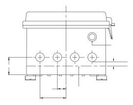
**NOTE:** Holes shown in Figure 5 are drilled at 7/8" for 1/2" trade size conduit. If larger conduit are needed, the minimal 1/2" clearance must be maintained between the hole's bottom to the control board inside the Blue Genius™ box.
