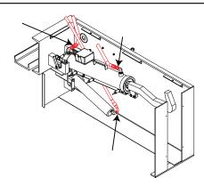
9. Install the J-box on the right-side wall with the pre-installed screws and rubber inserts are provided.
