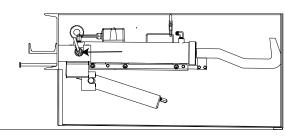
Apply Blue LOCTITE® 242 to the necessary bolts then bolt the hook cylinder and tilt cylinder into place on their trunnion carriages
