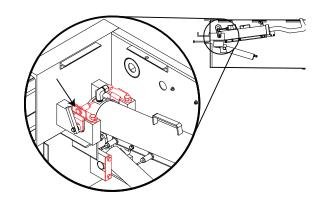
Connect the hoses from the cylinders to the RVR303 Powerpack.
