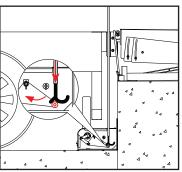
NOTE: The truck / trailer is NOT restrained if the arm is not fully vertical and the communication lights do not change colour as described above. Do a visual inspection to confim that the ICC bar is securely restrained before proceeding with loading / unloading.
