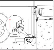
NOTE: If the ICC bar is applying pressure to the restraint arm, it may be necessary to have the driver back up the vehicle before releasing the arm.
