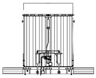
**Rail Dock Leveler** These levelers involve a variation on the vertical leveler and are used to service rail cars. They are usually mounted on a sliding rail that allows them to move horizontally along the rail track. They may either be manually or hydraulically moved along the track and are typically hydraulically operated levelers.
