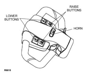
Figure 2-3 Pushbutton Switches
