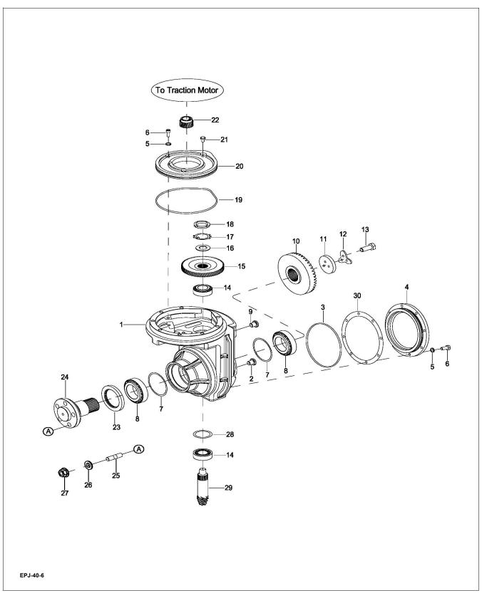
Figure 12-6 Transmission Used up to Serial # E2219364
