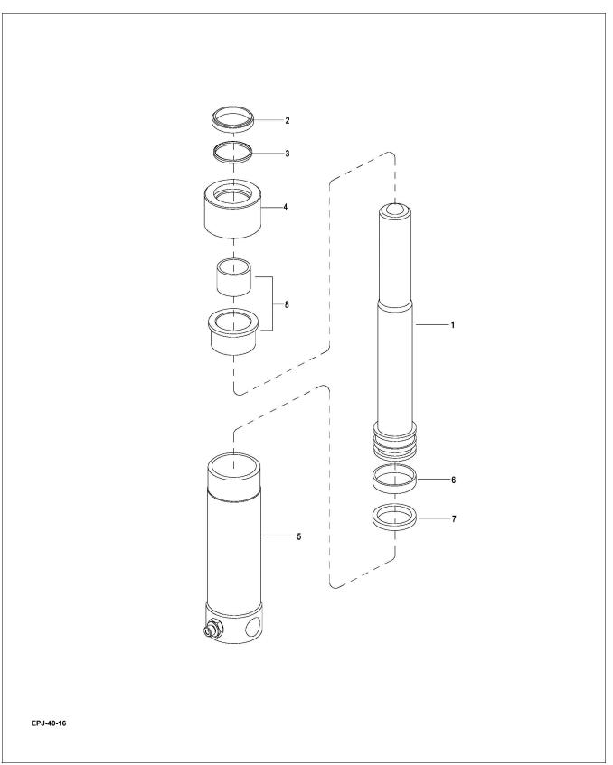
Figure 12-16 Lift Cylinder
