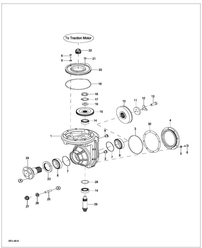
Figure 12-6 Transmission Transmission Used up to Serial # E2219364
