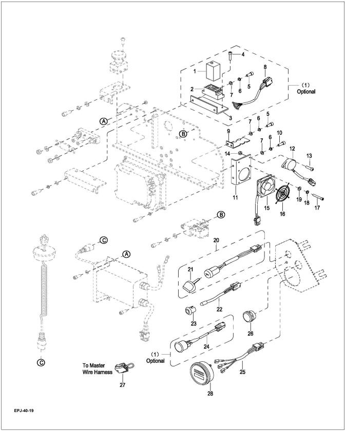
Figure 10-2 Electrical Components (Sheet 2)
