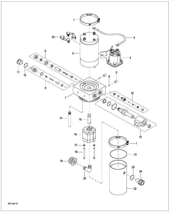
Figure 9-2 Pump & Motor Assy
