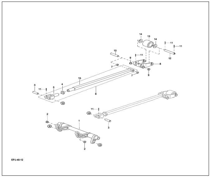
Figure 8-2 Lift Linkage Assembly
