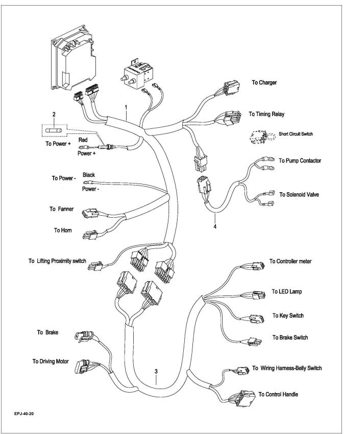
Figure 12-21 Wiring Harness
