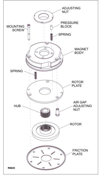
Figure 6-1 Brake Assembly
