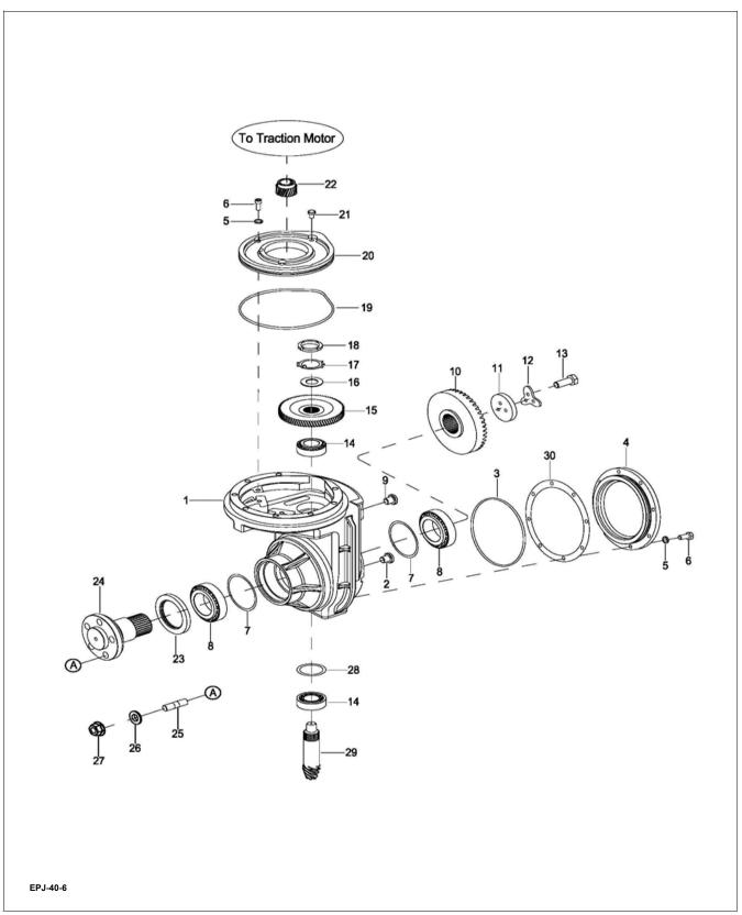
Figure 12-7 Transmission Used from Serial # E2219365
