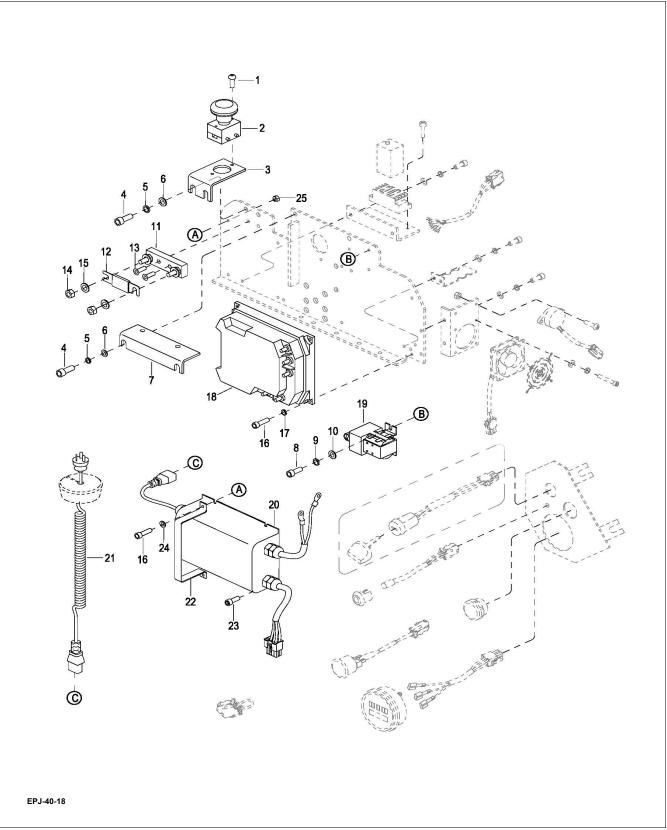
Figure 12-19 Electrical Components (Sheet 1)
