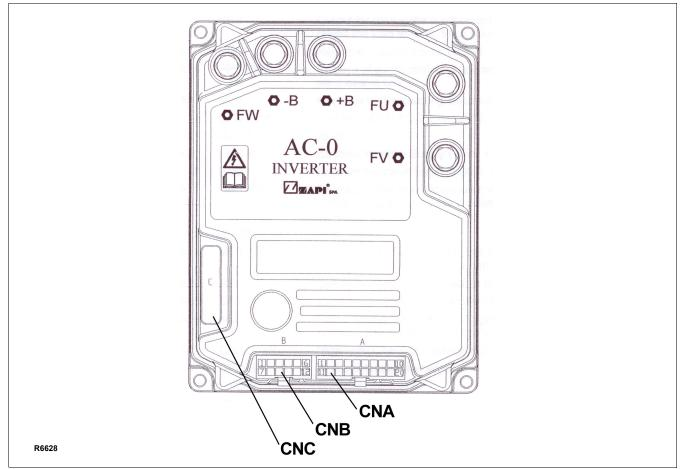
Figure 4-6 Zapi Controller Connections
