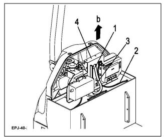
Figure 3-3 Controller Board Removal
