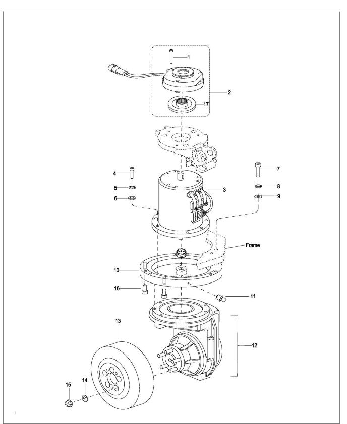
Figure 12-5 Transmission Motor, Brake Mounting
