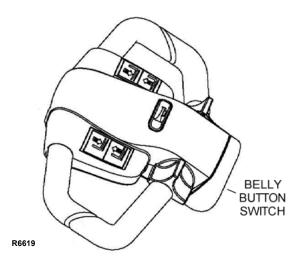
Figure 2-5 Belly-Button Switch
