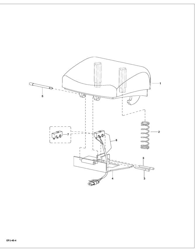
Figure 12-4 Emergency Reverse Switch Assembly
