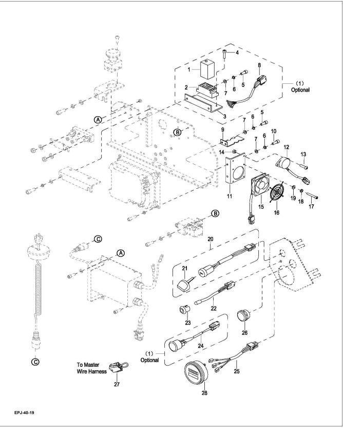
Figure 12-20 Electrical Components (Sheet 2) - Continued
