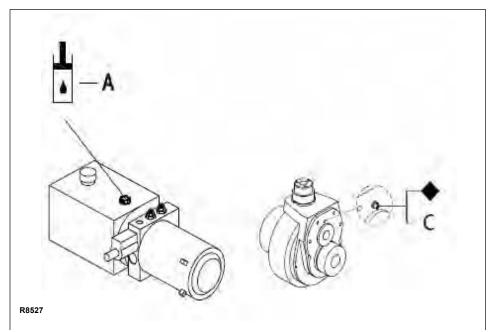
Figure 9 Lubrication Diagram
