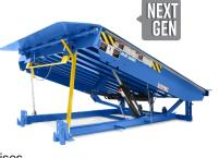
and the lip moves smoothly into the locked position. Simply 'walk the deck' to lower it onto the truck bed. The mechanical dock leveler hold-down system reduces cross-traffic bounce, lowering the risk of cargo and equipment damage.
